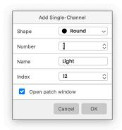
When you add any DMX fixture you will see a window that allows you to select the number, shape and, in some cases, type. There's also a check box to open the patch window if you wish to assign a DMX address right away. This can be done later in the Properties panel when a fixture is selected.
