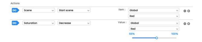
In summary our T-C-A trigger occurs at 12.00 everyday IF port 1 is pressed. When it's 12.00 and port 1 is pressed the Red scene in our Global zone activates at 55% saturation. You can see the complete trigger in the image below.
