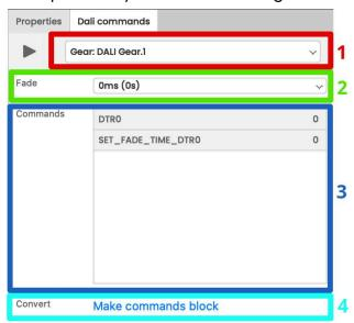
The dropdown at the top of this window (1) allows you to select which DALI gears the command block will affect. Each gear will be individually listed but you also have the option to set it to a Group or Broadcast. When you set a Command block to Broadcast a new dropdown menu will appear to the right, here you can select which DALI Bus the command will broadcast to. Selecting a group will send the command to all gears in a DALI group.
