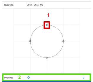
The shape in the center (a circle in this case) represents the motion your moving head will make. By dragging and stretching the dots around the shape (1) you can manipulate the motion your moving head makes. You can add anchor points just like with the LED strip fixture type, this allows for truly unique movement.
